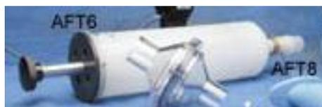
**Calibration 2** – Do 5 push-and-pulls with plunger: 1 sec push or pull, then 2 sec between each.
